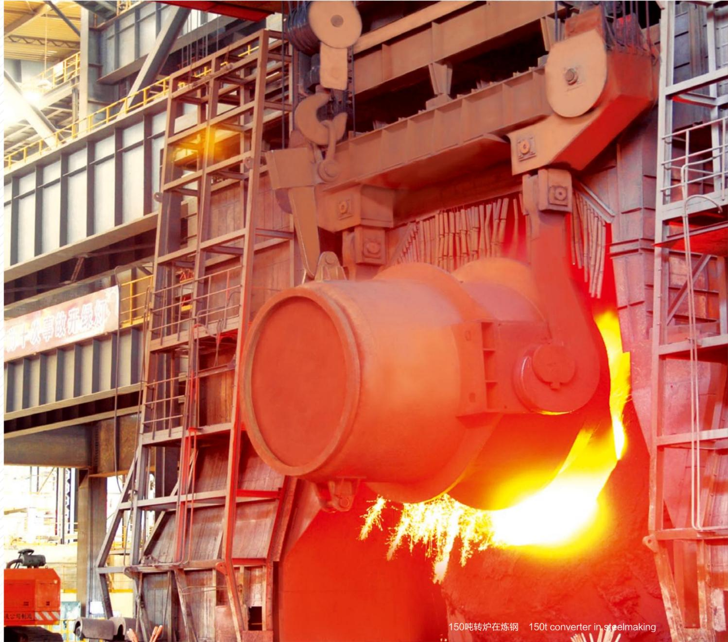
150吨转炉在炼钢 150t converter in steelmaking
