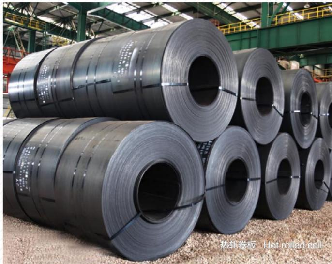
热轧卷板 Hot-rolled coil
