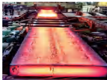
475mm板坯铸机 475mm Slab Caster
