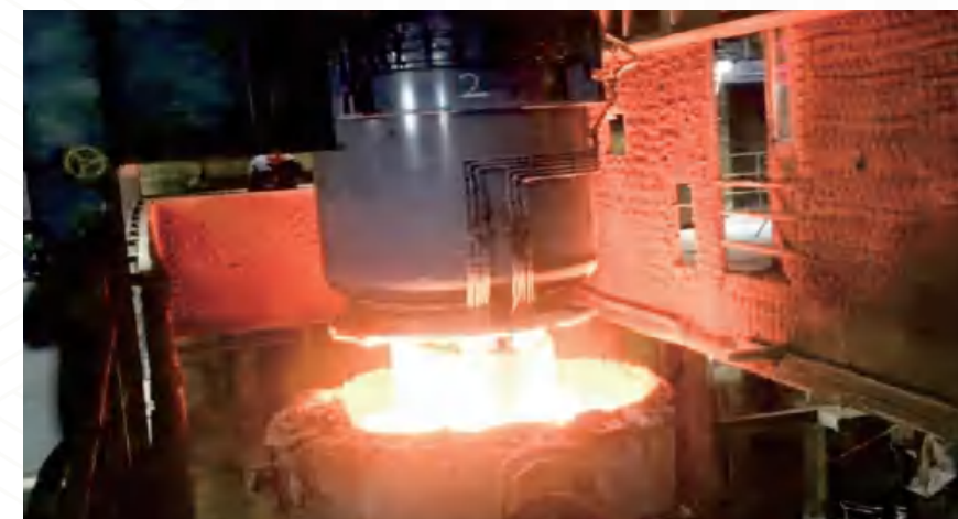
120吨RH真空精炼炉 120-ton RH Vacuum Refining Furnace
