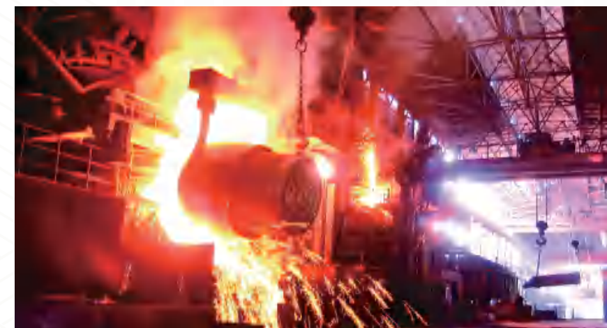
120吨顶底复吹转炉 120-ton Top/Bottom Combined Blowing Converter
