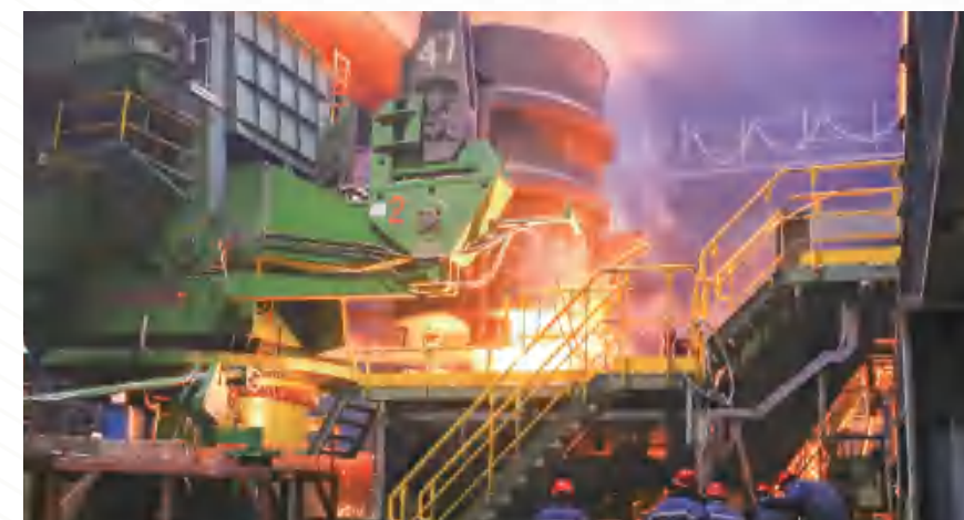
475mm板坯铸机 475mm Slab Caster
